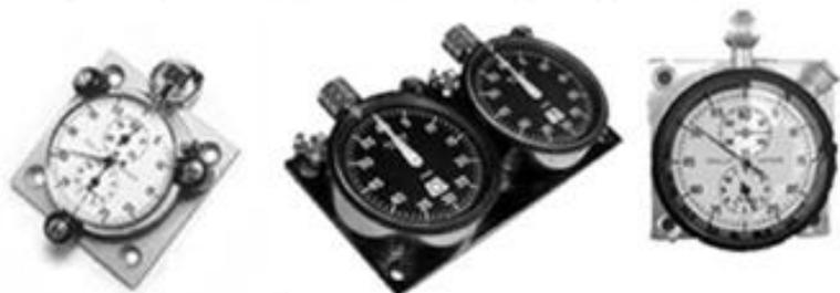
All kinds of analog chronometers are allowed to be used in the car. Whether mounted in the car or hand held.
